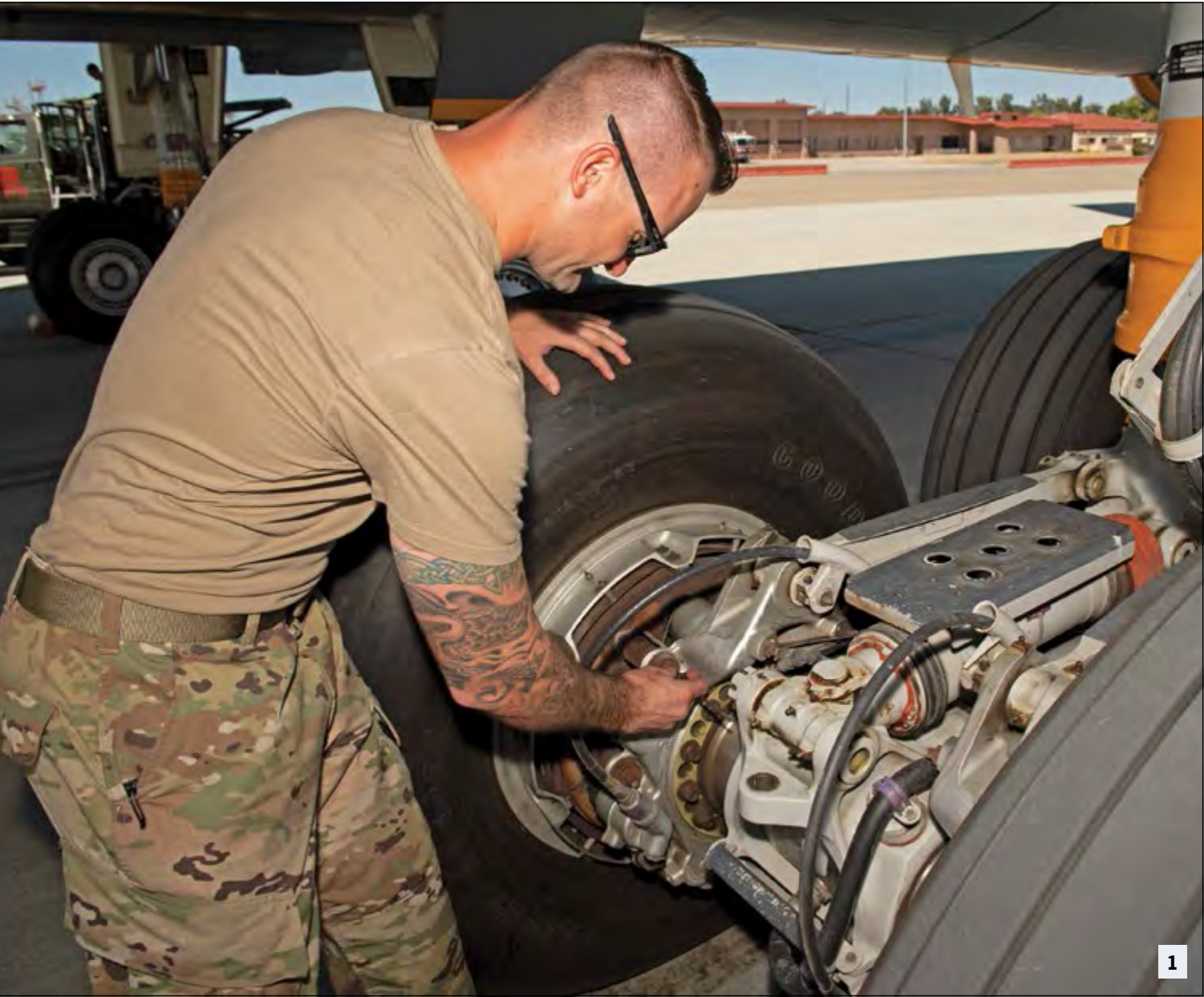
1) U.S. Air Force Senior Airman Jacob St. George, 660th Aircraft Maintenance Squadron dedicated crew chief, checks the brake piston on his KC-10 Extender July 13 at Travis Air Force Base, California. The purpose of the dedicated crew chief program is to provide continuity and accuracy by assigning ownership to each aircraft. St. George signed off the aircraft forms with zero discrepancies before flight, deeming the flight as a “Black Letter.” 2) St. George fills out aircraft forms post flight for a KC-10 Extender July 13 at Travis. 3) St. George checks the oil level of the constant speed drive on a KC-10 July 13 at Travis. The constant speed drive works similarly to the transmission in a car.
