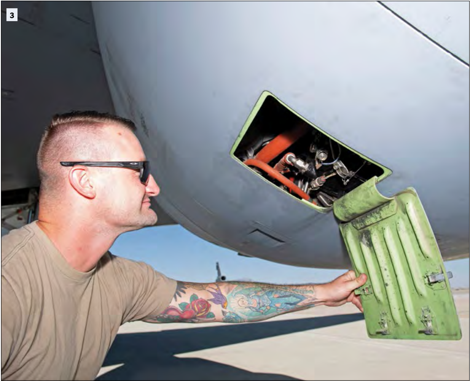
1) U.S. Air Force Senior Airman Jacob St. George, 660th Aircraft Maintenance Squadron dedicated crew chief, checks the brake piston on his KC-10 Extender July 13 at Travis Air Force Base, California. The purpose of the dedicated crew chief program is to provide continuity and accuracy by assigning ownership to each aircraft. St. George signed off the aircraft forms with zero discrepancies before flight, deeming the flight as a “Black Letter.” 2) St. George fills out aircraft forms post flight for a KC-10 Extender July 13 at Travis. 3) St. George checks the oil level of the constant speed drive on a KC-10 July 13 at Travis. The constant speed drive works similarly to the transmission in a car.
